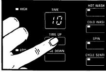
When a CYCLE Selection is touched, the amount of wash agitation time will appear in the TIME Display. The wash agitation time which appears is the recommended time for that cycle (for normally soiled items). If more or less time is desired, touch the TIME UP or TIME DOWN pad until the desired amount of time is showing in the TIME Display, before the end of the first fill.
